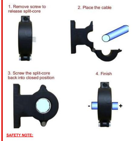
Although the voltage(s) directly connected to this instrument and its internal voltages are low, the cable running through the split core may be carrying dangerous high voltage. For this reason, this product should be installed by a competent person. If the unit fails to operate correctly then first check that the wiring is correct. Under no circumstances is the unit to be taken apart to gain access to internal circuitry for any reason whilst it has a live cable through the core.
