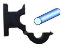
Screw the split-core back into closed position
