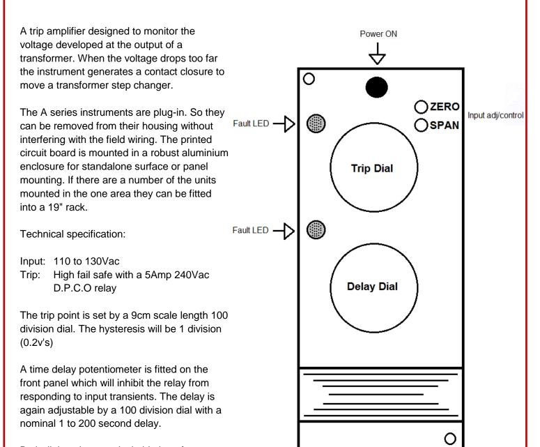
Both dial settings are lockable by a front fascia M4 screw. One LED shows that the input has seen a trip condition and a second showing that the time delay period has been exceeded and that the relay has changed state.
