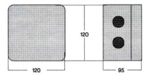
This mounting is available in fibre filled plastic; or diecast aluminium when RFI protection is required. Fixing holes should be drilled on 102mm by 92mm centres.
