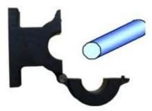
Screw the split-core back into closed position
