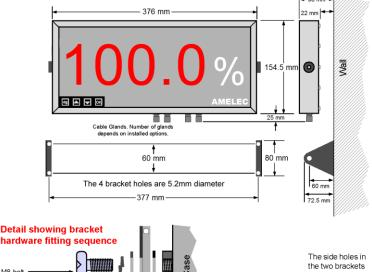
The side holes in the two brackets are 8.5mm dia. to accept M8 bolts.
