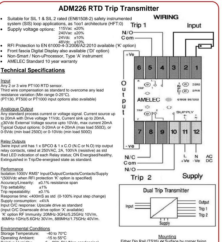
Either Din Rail (TS35) or Surface by corner fixing holes as standard.
