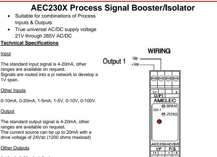
0-10mA, 0-20mA, 1-5mA The output current is configured as a source port as standard.
